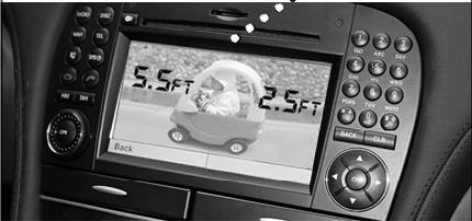
*Hideaway Interface Module and Stealth-in-bumper Camera make for a clean and obscure installation. Camera is seen automatically when Reverse is engaged.*
